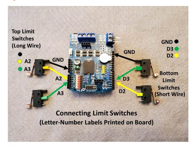
(1) The photo shows the connection on the Rover Driver Board for D2, D3, & GND to the Top Stepper Limit Switch wires and are marked as GEEN, YELLOW, & BLACK sleeves.
